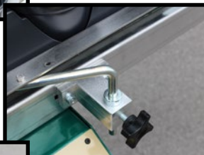
Guide rail adjustment
