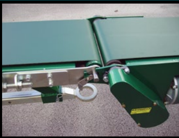
Conveyor to conveyor interlocking system
