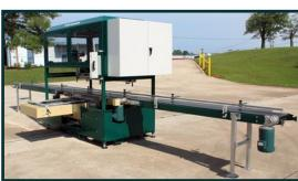
The B&L PlugPlanter M or S model offers fast accurate planting, quick change-over and CNC operating system for one of the easiest, quickest setups available. Quick-change grippers for easily switching plug size and push-up pins to ensure soft or young plugs are extracted and planted without damage. The PlugPlanter gives you flexibility to use your plug tray widthwise or lengthwise on the same machine to match container and plug tray count in the most efficient way.
