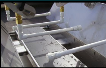
"T" bars standard with interchangeable nozzle system
