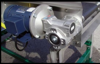
Direct drive gearboxes for low maintenance.
