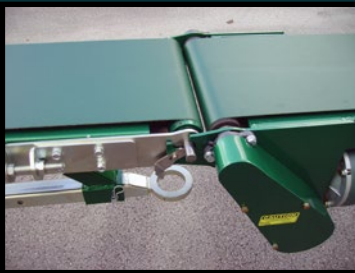
Conveyor to conveyor interlocking system
